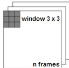
Fig. 1. Schematic representation of algorithm for calculating the contrast in the tLASCA method.
